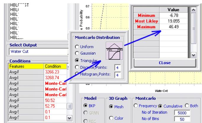
**Figure 10.** Assigning pdf to specific parameters in SRM.
