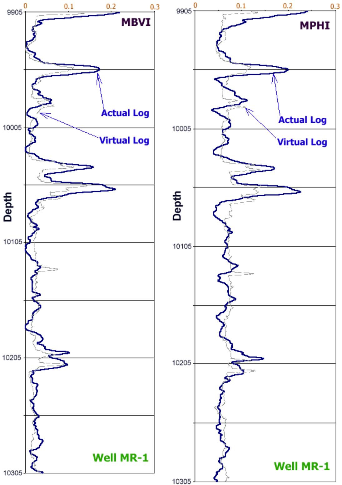
Figure 5. Actual and virtual magnetic resonance logs for well MR-1 along.
