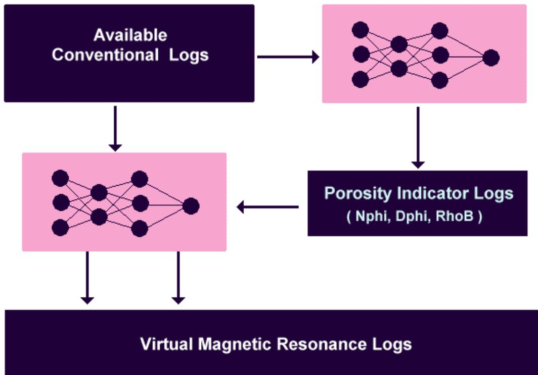
Figure 2. Schematic diagram of the process for developing virtual magnetic resonance logs.
