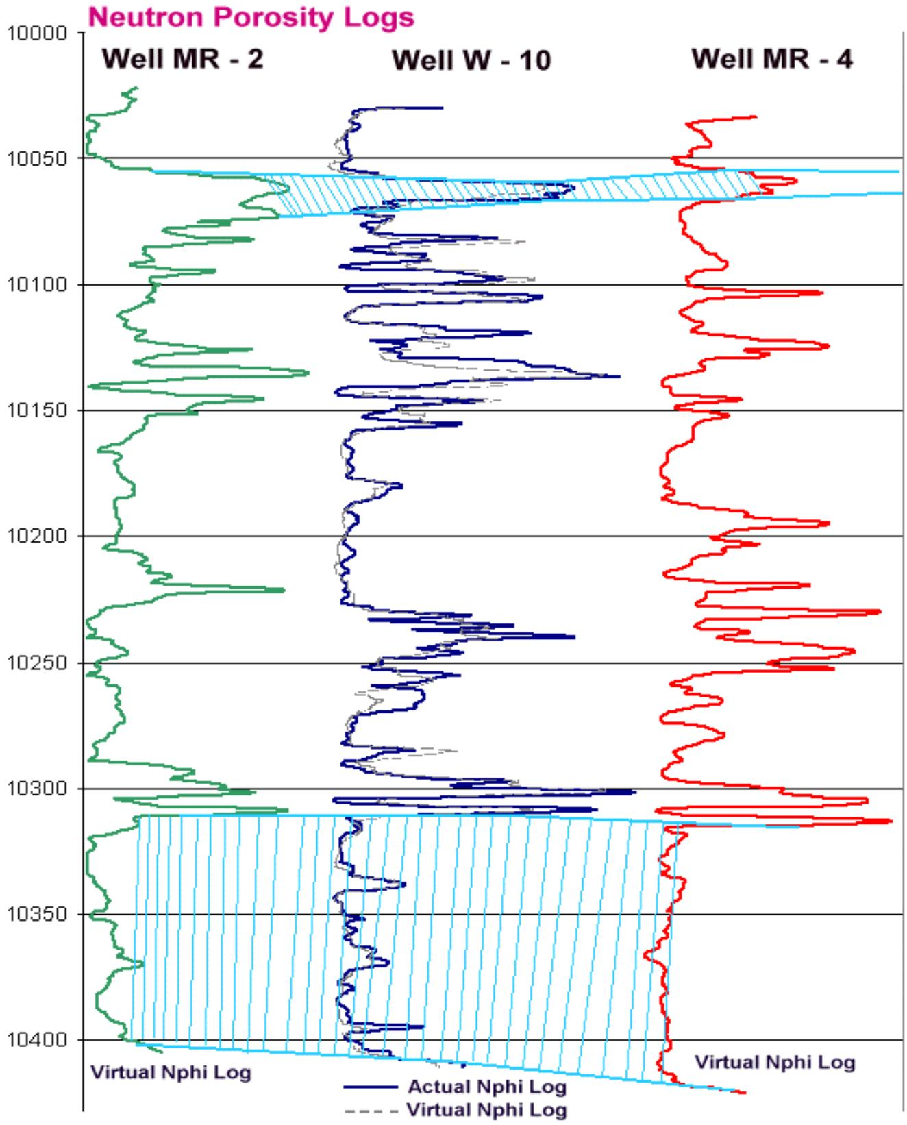
Figure 4. Actual and virtual neutron porosity logs for well W-10 along with virtual Nphi for wells MR-2 and MR-4.
