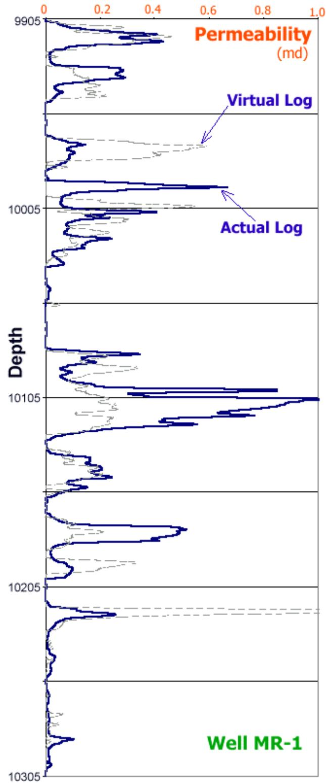
**Figure 6.** Actual and virtual magnetic resonance permeability logs for well MR-1 along.
