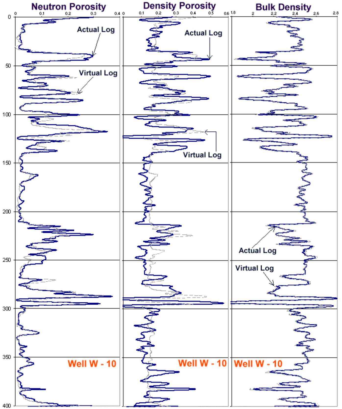
Figure 3. Actual and virtual porosity indicator logs for well W-10.
