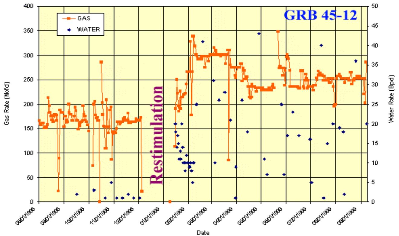
**Figure 8.** Gas and water production before and after restimulation for well GRB 45-12.
