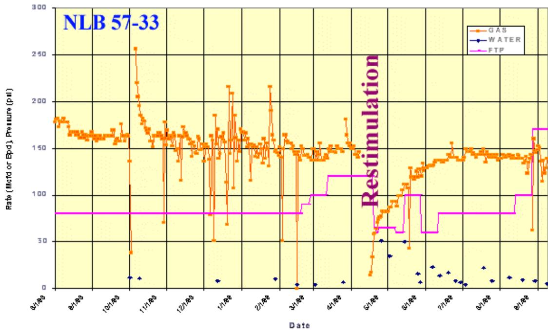
Figure 10. Gas and water production before and after restimulation for well NLB 57-33.
