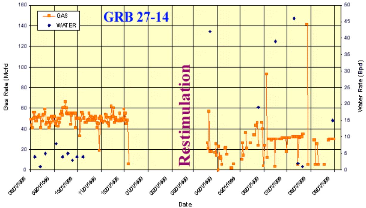
Figure 9. Gas and water production before and after restimulation for well GRB 27-14.
