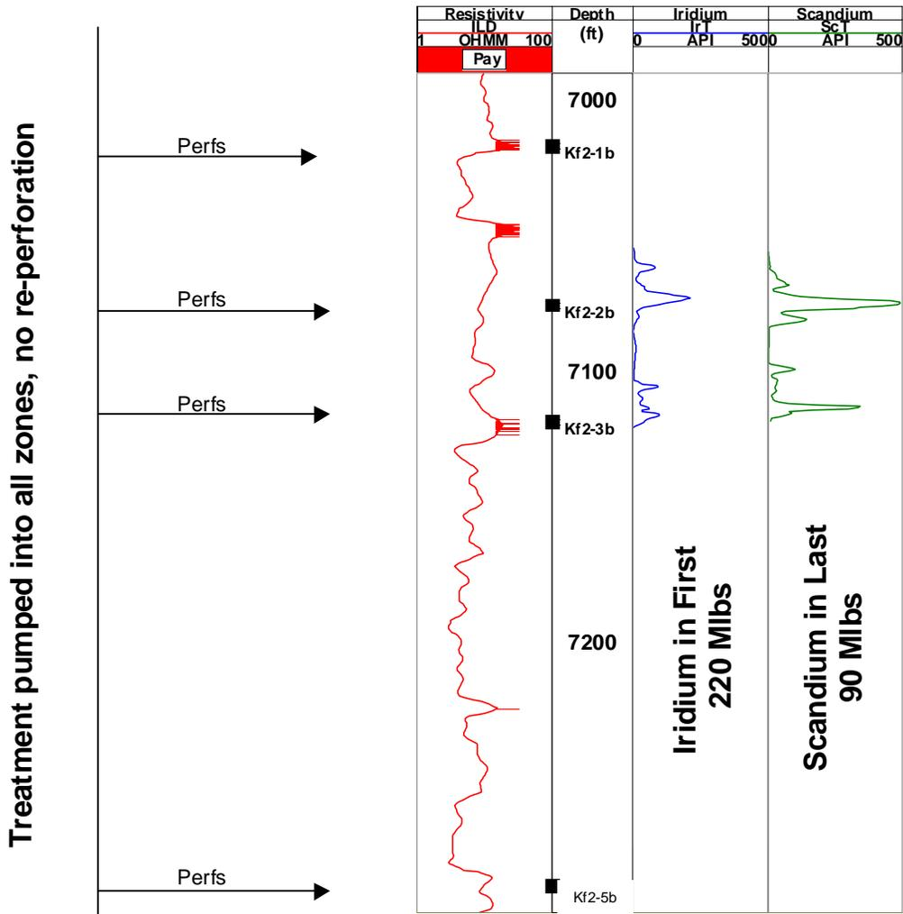
Figure 9: Post-Treatment Radioactive Tracer Survey, GRB 45-12
