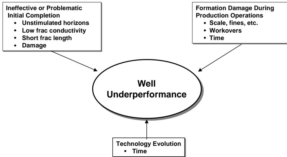
Figure 3: Potential Sources of Well Underperformance
