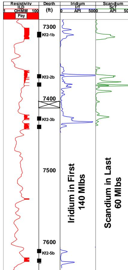
Figure 11: Post-Treatment RA Tracer Survey (GRB 27-14)
