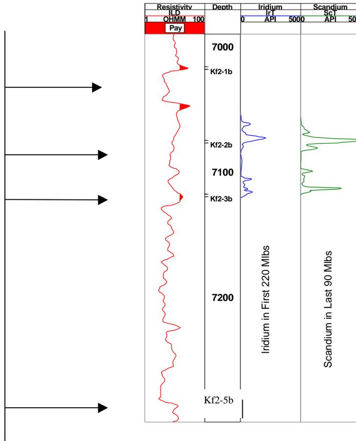
**Figure 9 - POST-TREATMENT RADIOACTIVE TRACER SURVEY, GRBU 27-14**
