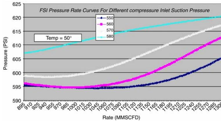
**Figure 13** Rate versus pressure curves for FSI at 50° Temperature and different Compressor Inlet Suction Pressures
