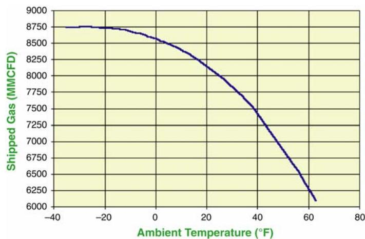
**Figure 3** Shipped gas versus ambient temperature in 2001
