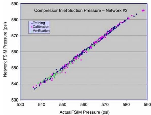
**Figure 12** Cross plot for Compressor Inlet Suction Pressure, network model #3
