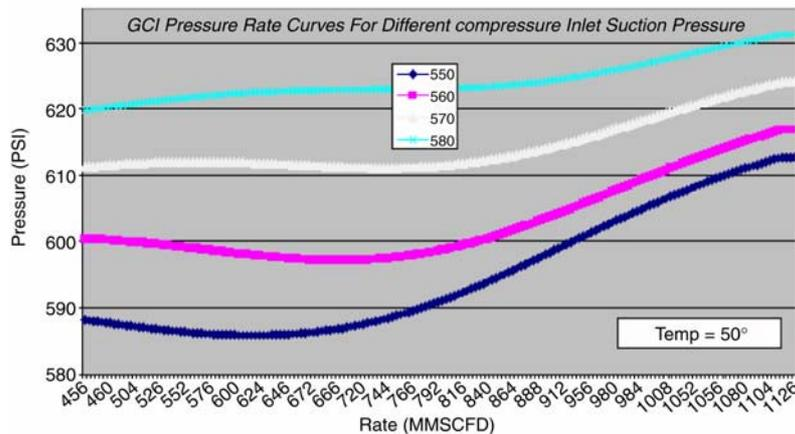
**Figure 14** Rate versus pressure curves for GCI at 50° Temperature and different Compressor Inlet Suction Pressures
